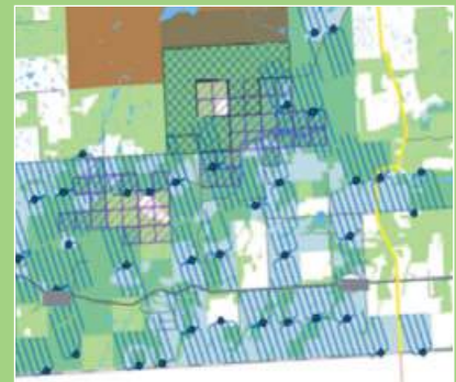
Well pad placement using four constraints: native prairie; protected areas; watercourses; and residences
